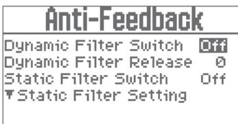
3. Configurar " Static Filter Switch " en " On " .
